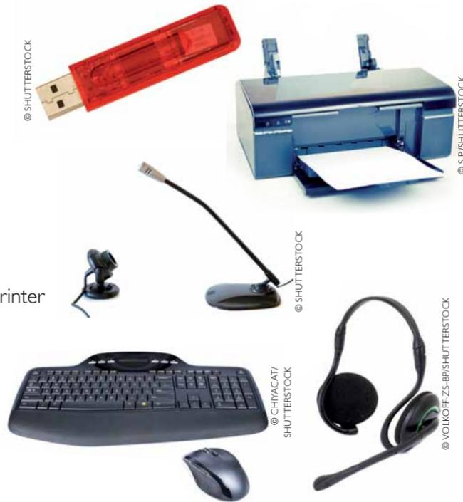
An input device is a peripheral that lets you send information or commands to the computer — for example, the keyboard.
